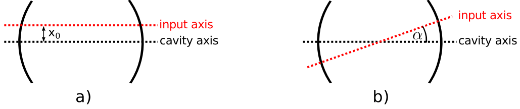
Figure 10.2: Different possible misalignments of an optical cavity. a) Constant x displacement of the input beam optical axis with respect to the cavity axis. b) Relative tilt between the input optical axis and the cavity axis.
