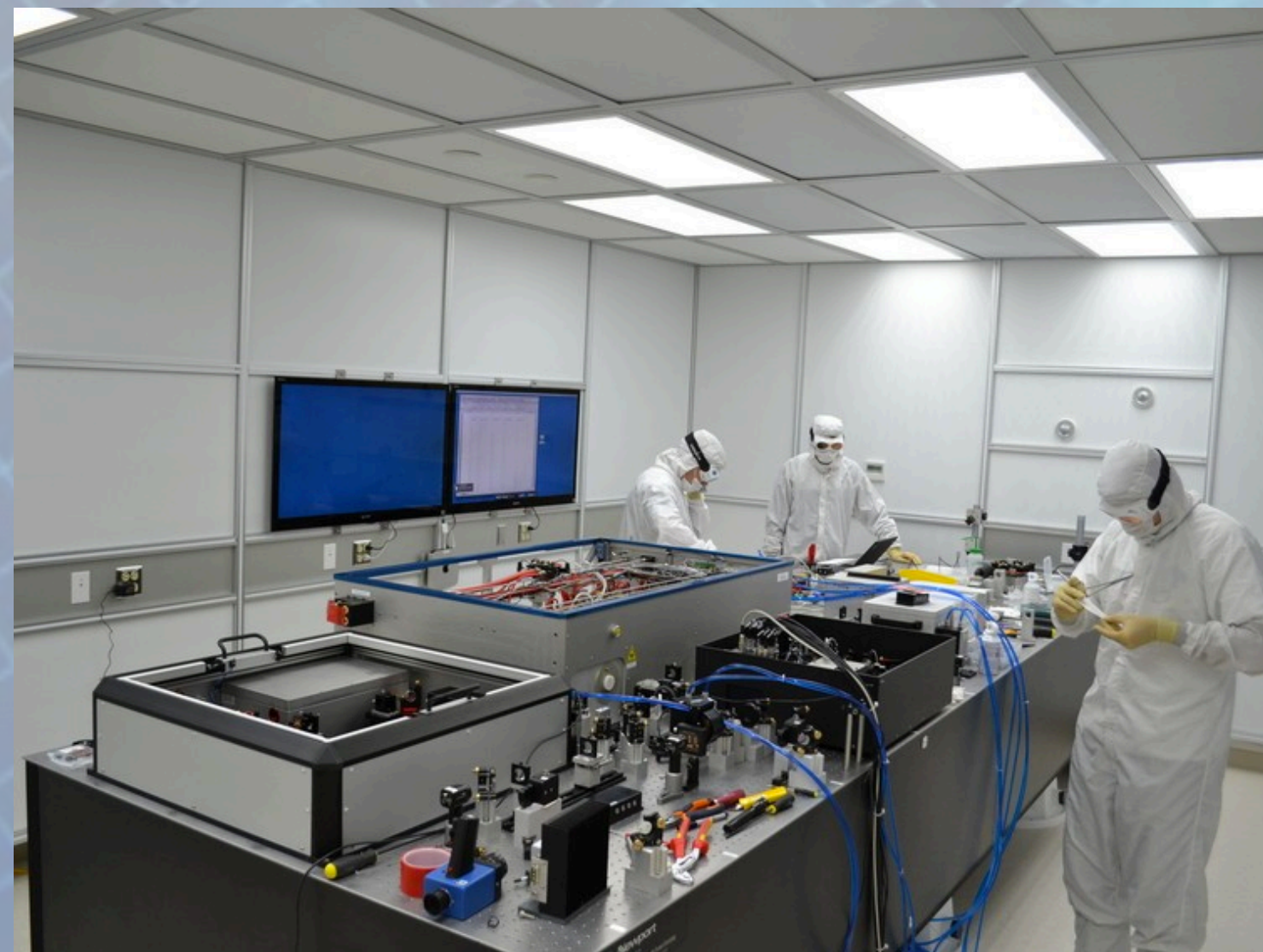
A new laser system was installed and top laser power boosted from 4.5 W to 125 W [3, 8]. Image from [9].
