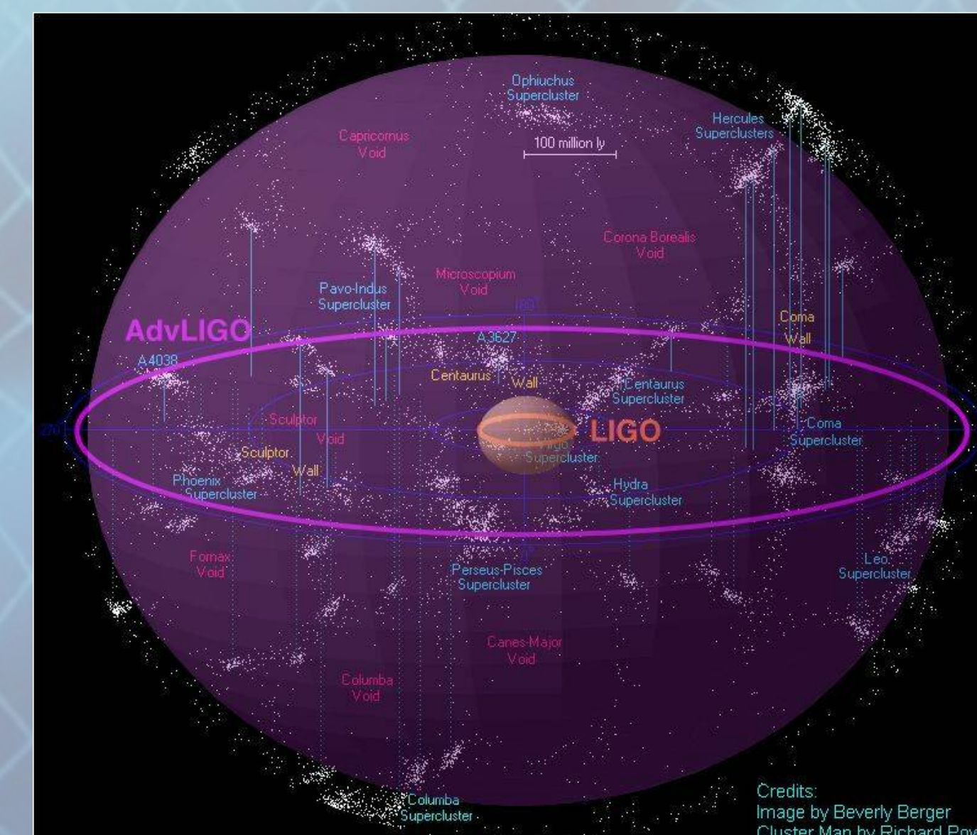
The above diagram shows the volume of space for which Initial LIGO was able to measure gravitational waves produced by the inspiral of two neutron stars. Once the detectors reach design sensitivity, Advanced LIGO will be able to see far enough to make frequent detections. Image from [13].
