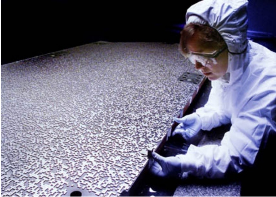
Swift Burst Alert Telescope: Coded mask, 50% occulted by 5x5mm Pb tiles
