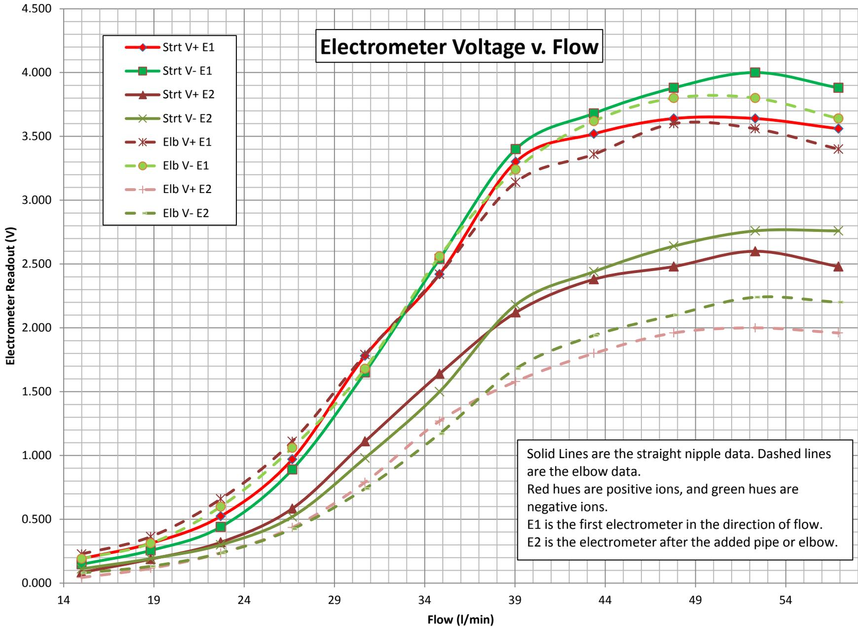
Solid Lines are the straight nipple data. Dashed lines are the elbow data.
