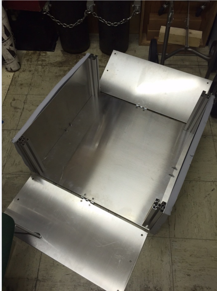
Lid construction: more aluminum machining, foam cutting, and beam attachment
