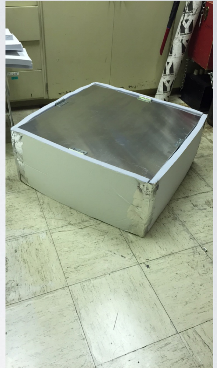
Lid construction: more aluminum machining, foam cutting, and beam attachment
