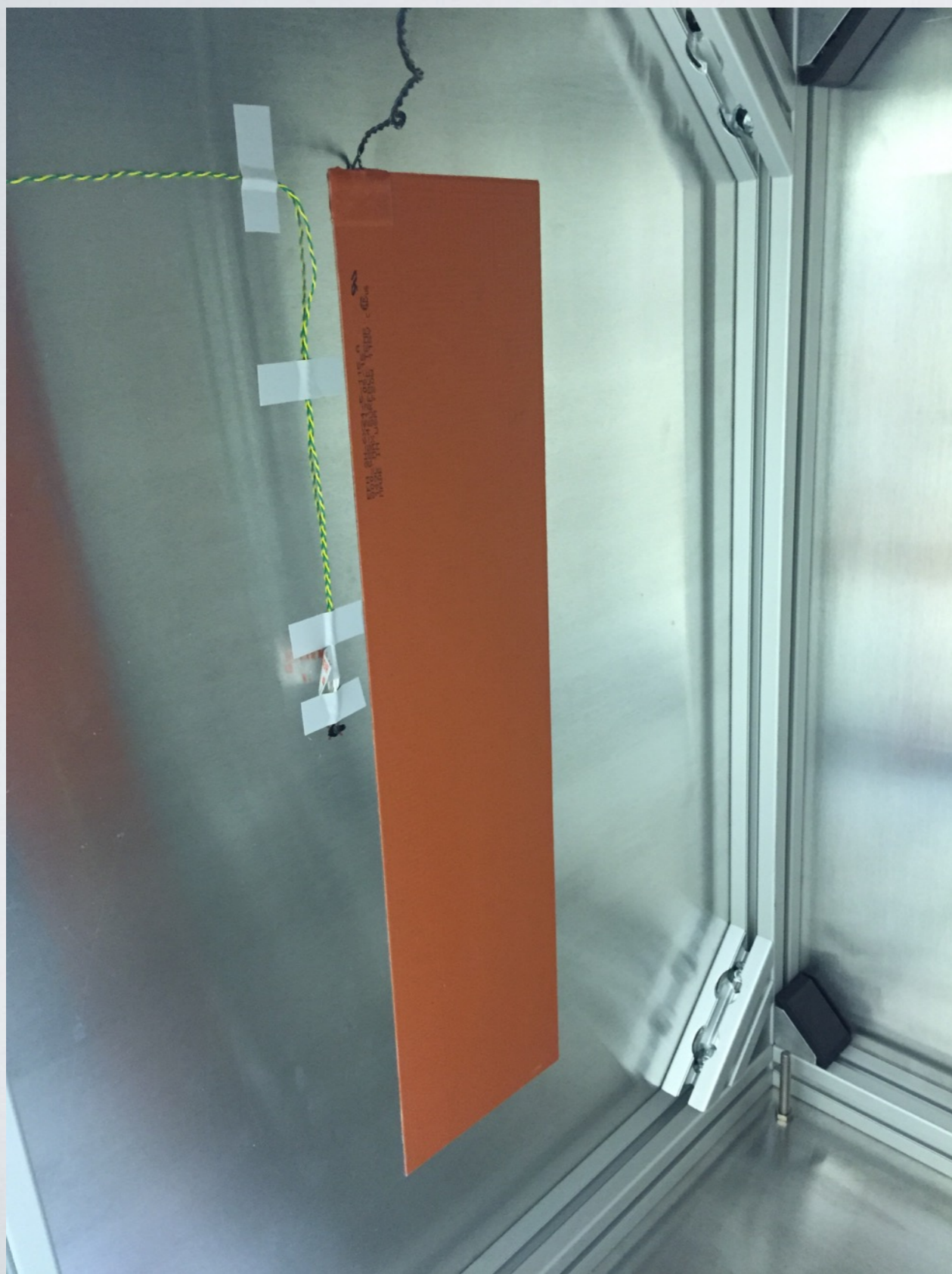
Full-size heater, and thermistor attached with epoxy
