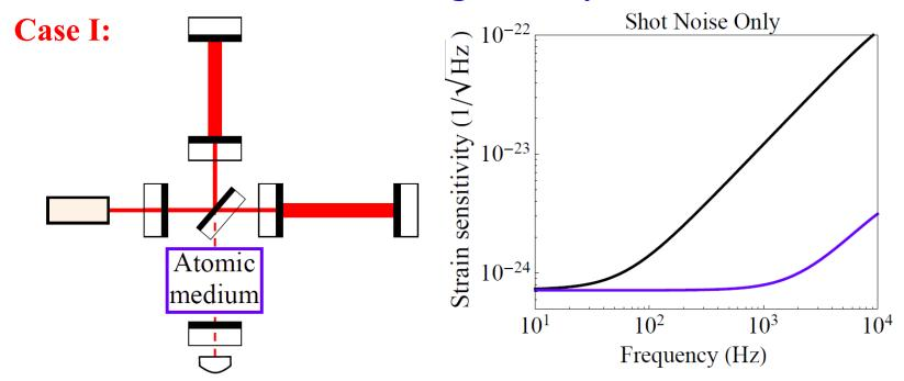
**Principle:** Negative dispersion to compensate propagation phase
