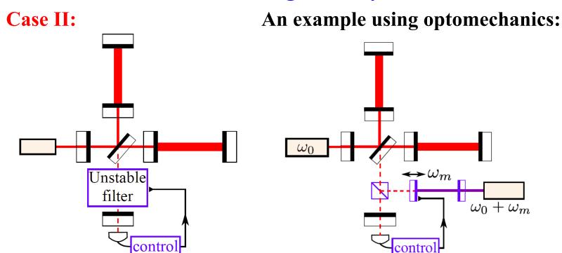
**Challenge:** thermal noise from mechanical oscillator (optomechanics)
