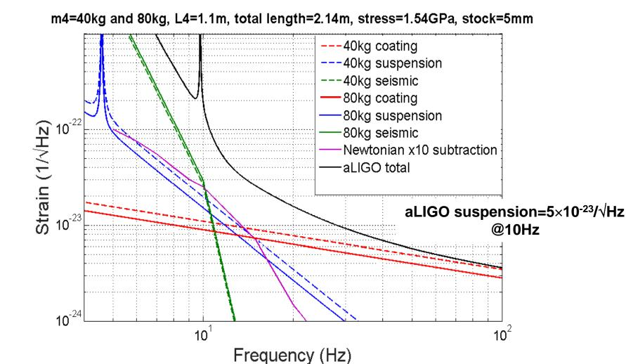
• Longer suspensions (final stage 1.1m) and higher stress offer further improvements for both 40kg and 80kg
