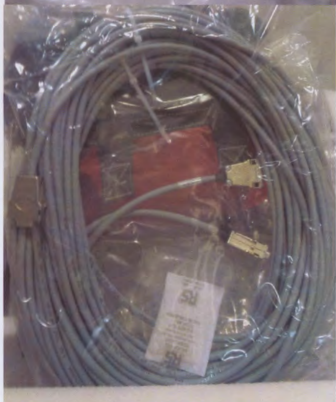
CHILLER COMMUNICATION CABLES: xtal chiller_RS232, diode chiller_RS 232
