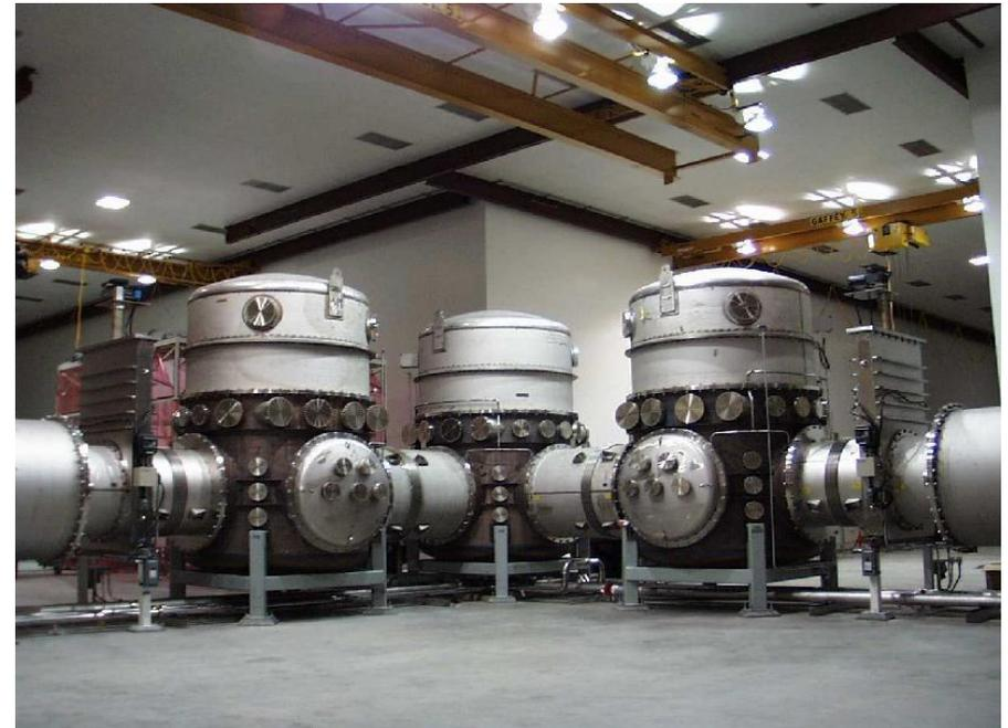
All optical components must be in high vacuum, so mirrors are not “knocked around” by gas pressure
