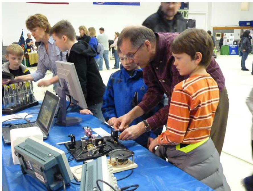
Figure 4.6: Aligning 'baby LIGO' – a small Michelson interferometer
