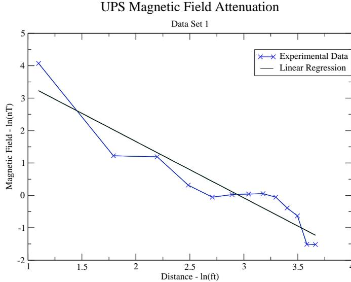
Figure 5: UPS Magnetic Field Attenuation
