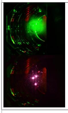
Image with the PCal camera with ALS green laser light resonant in the arm cavity. Residue at the perimeter of central alignment layer is clearly visible. There are also three large bright scattering locations.
