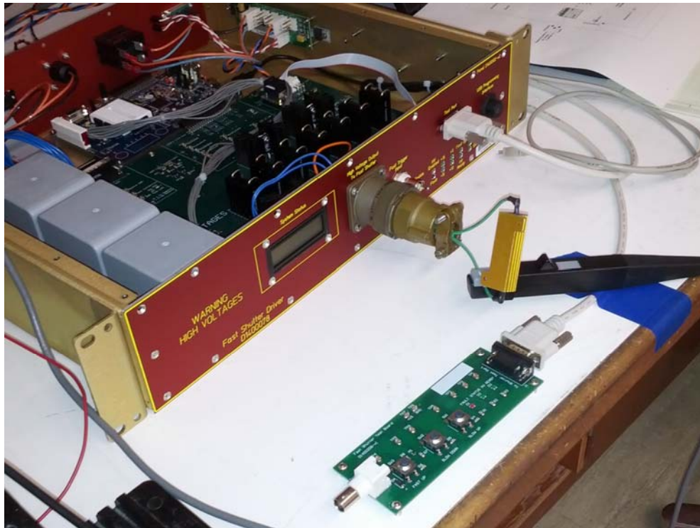
Figure 2 shows the dummy load with integral short, clamp-on current probe, and test board
