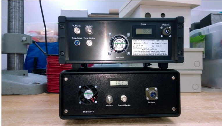
Figure 13) the back of the laser chassis. The smaller chassis is on top and has external TEC controls
