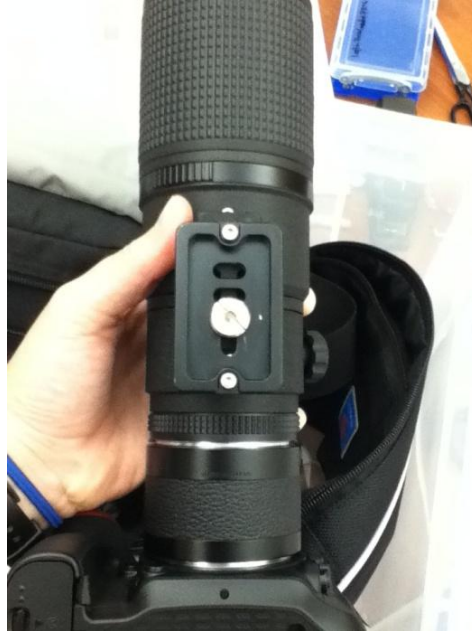
Attaching the Tripod Mount to the Lens
