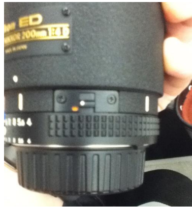
Unlocked Position of the Switch that Controls the Aperture Band
