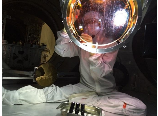
Figure 15. Painting a crust of First Contact around the sprayed First Contact on one of the large optics, one side of the beamsplitter optic (BS), see Figure 1.
