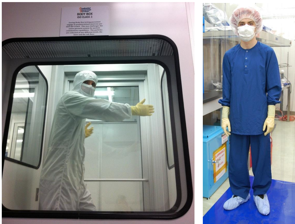
Figure 7. Body Box testing of cleanroom garb (LHS).
