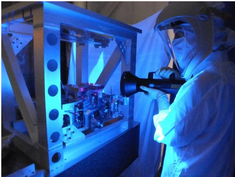
Figure 11. Black light inspection of assembly (LHS).
