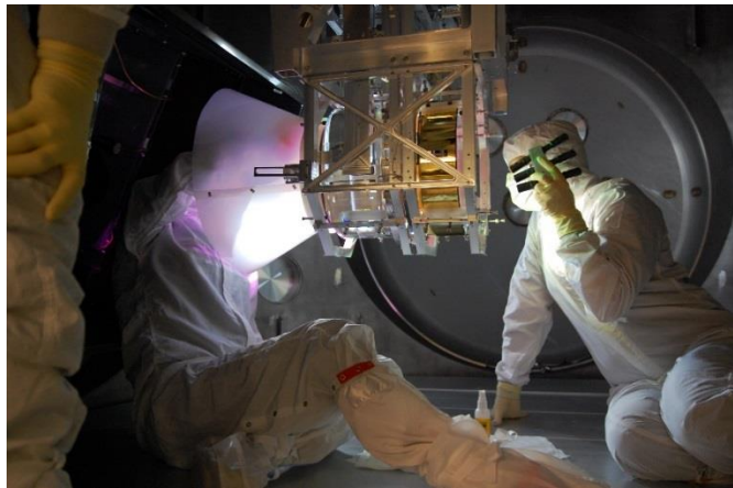
Figure 14. Spray application of First Contact on a large ITM optic (LHS).
