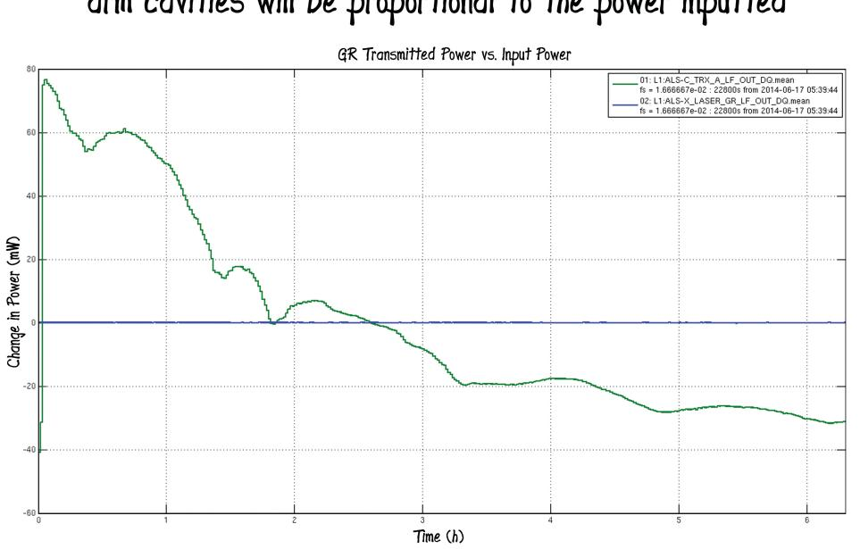
This plot shows the power from the laser vs time on June 17th. It can be seen that the power does not decay, so we can rule out the input power.
