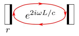
A positive feedback but with a phase delay:  $\phi = 2\omega L/c$
