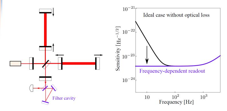
In principle, this allows for a shot-noise only sensitivity.
