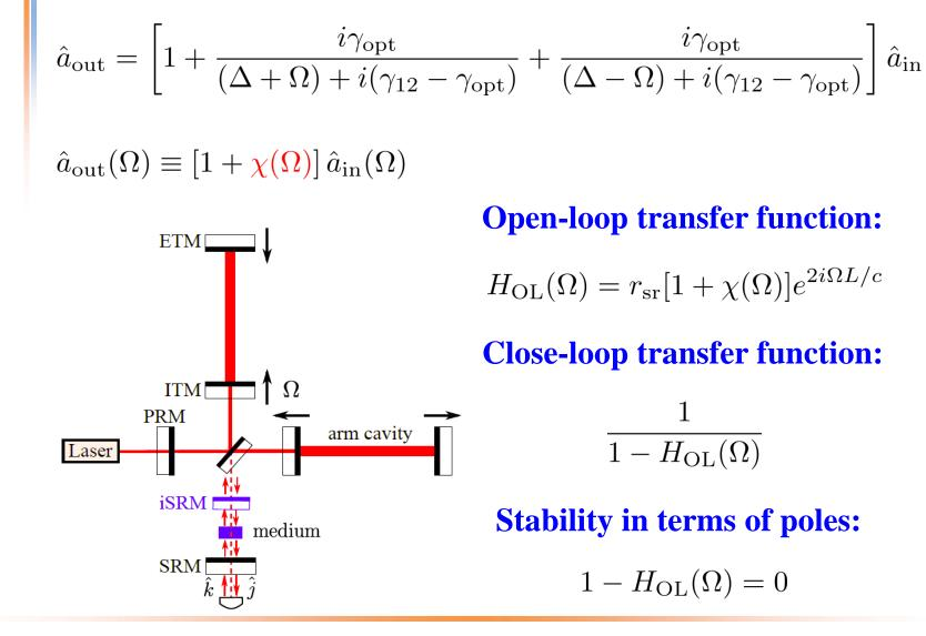
**Open-loop transfer function:**  $H_{\rm OL}(\Omega) = r_{\rm sr}[1 + \chi(\Omega)]e^{2i\Omega L/c}$
