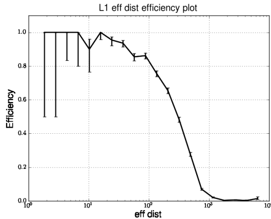
Figure 7.21: The efficiency at finding injections performed during S6a, the first analysis period of S6 (GPS time: 931035296-935798487), from all sets of EOBNRv2 waveforms enumerated above. These injections have been found in coincidence between L1 and at least one other detector during H1L1V1 time, at the end of the high-mass pipeline with Categories 1-4 of vetoes applied. The efficiency is plotted versus the binned injected effective distance (see Equation (7.7)) (in Mpc) of each waveform.
