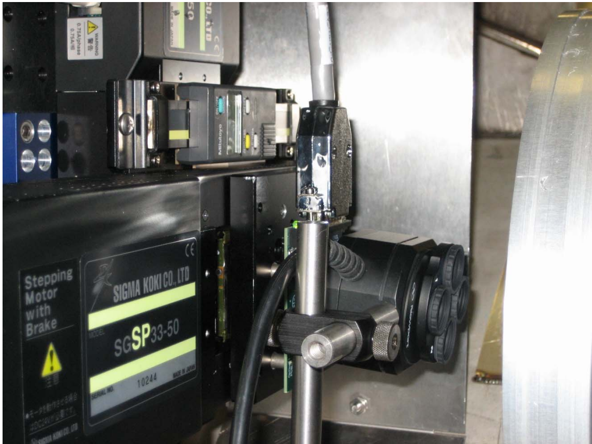
Profiler used to look at beam profile
