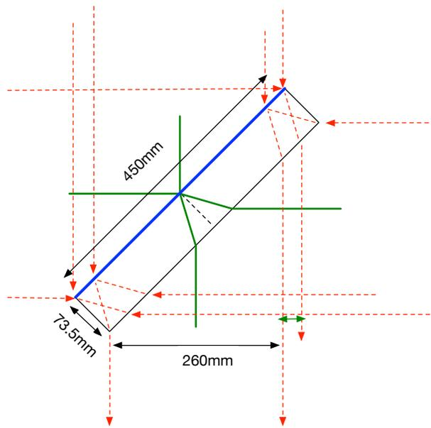
**Figure 3 BS geometry and clear aperture**
