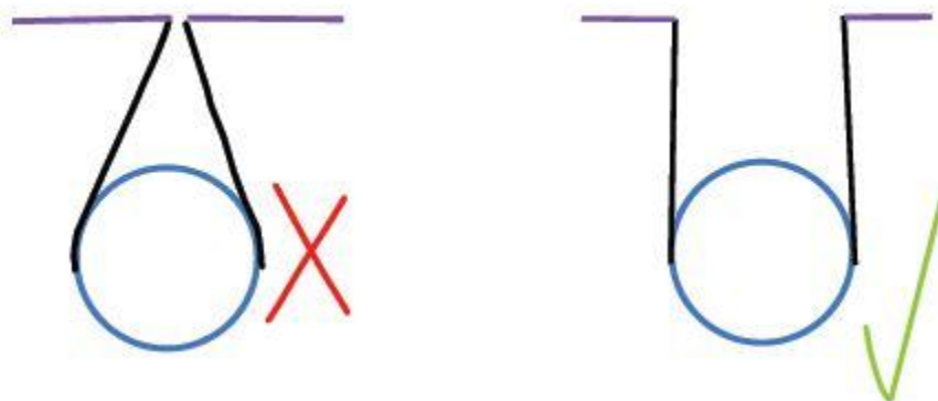
Figure 8: The example on the left is unacceptable, because the wires do not have a clean break-off from the prism, as they do in the example on the right
