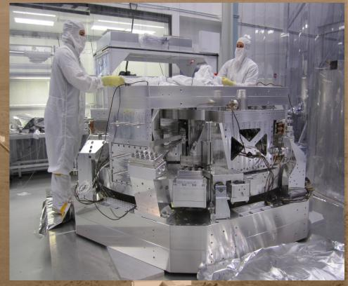
Hydraulic external (to the vacuum) pre-isolator stage and in-vacuum 2-stage active seismic isolation platform give horizontal attenuation > 10-10 at 10 Hz
