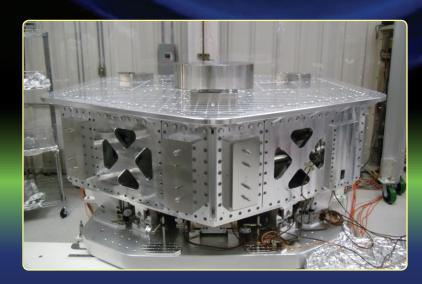
LIGO Vibration Isolation and Positioning Systems are designed to provide ultra-high levels of isolation over a very large frequency band. The platforms provide isolation from 0.1 Hz to several 100 Hz in six degrees of freedoms (3 translations and 3 rotations). Passive and active isolation are combined to obtain up to four orders of magnitude of attenuation in the control bandwidth.
