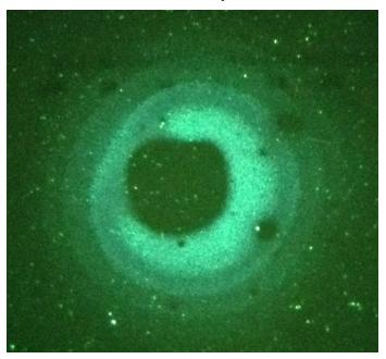
The dark field image from ITM11 shows one of the defect spots. The spots are typically  $\sim$ 1 mm in diameter measured from the edge of the visible ring structure.
