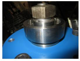
• Load cell values BSC HEPI load cell capacity → 3000 lbs
