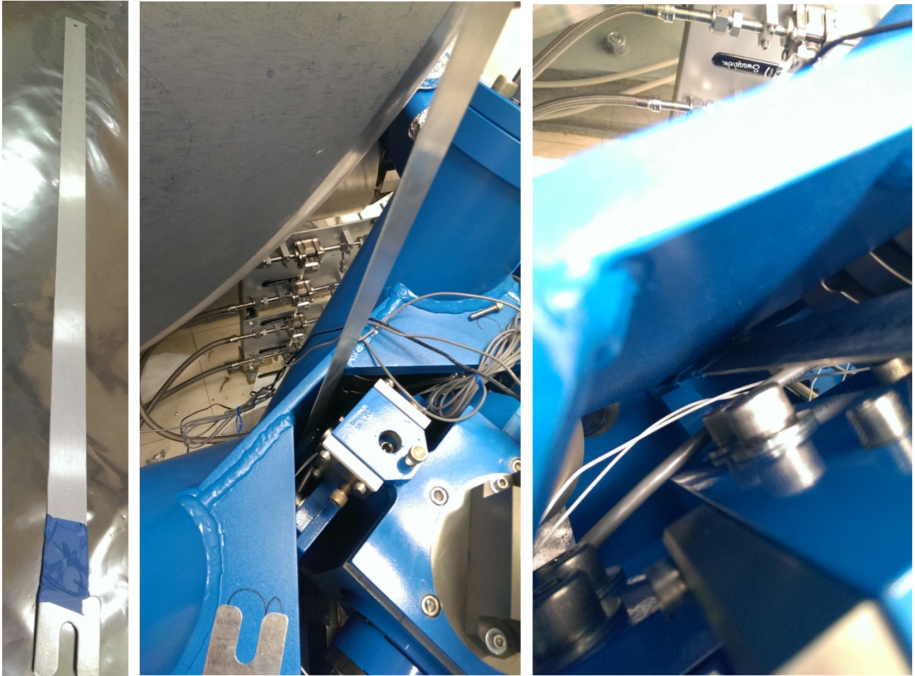
Figure 7: First gap to measure (on the first picture, we can see the tool used to measure that gap)
