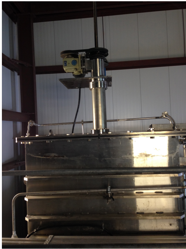
Figure 4: Upper trunk and stem. The drive housing has been removed to expose the motor, gearbox and leadscrew.
