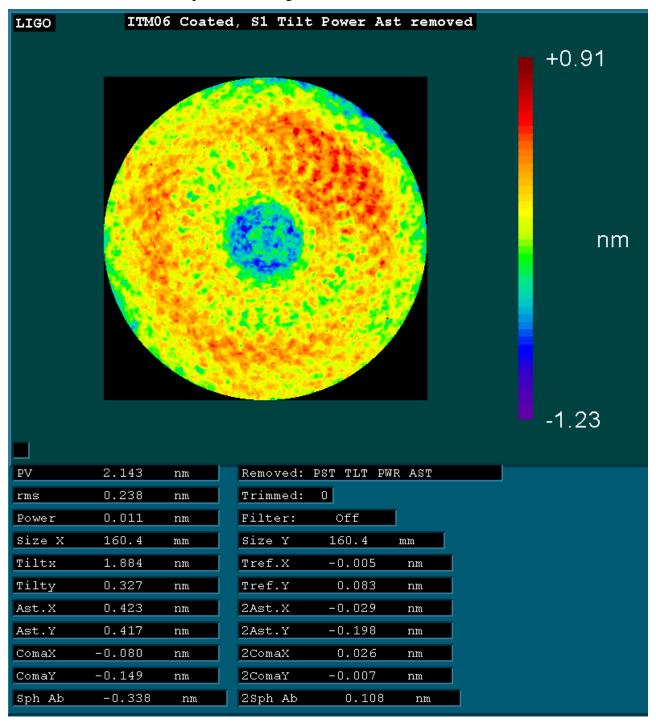
Amplitude of the spiral at R=40 mm, approximately 0.5 nm.
