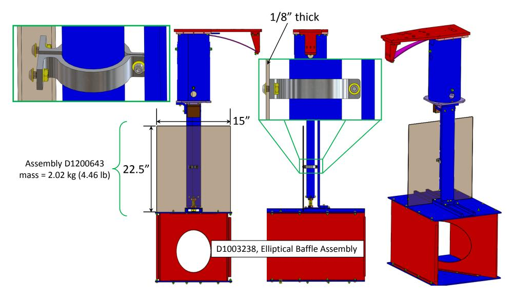
CONCEPT A1: A plate of tempered welder's glass (#14), clamped to the suspension post of assembly D1003238 (4.5lbm)
