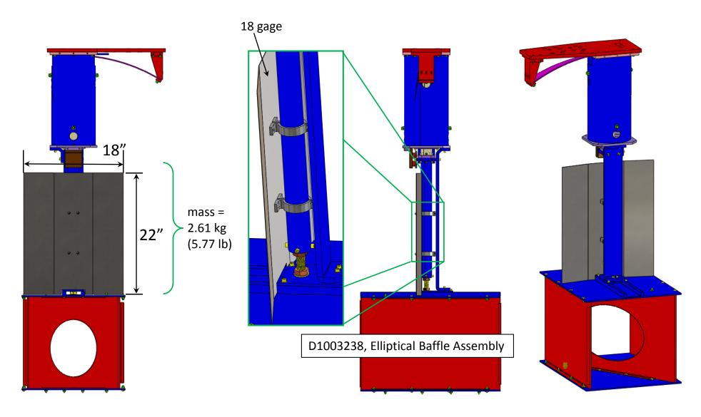
CONCEPT B1: Sheet metal (18 gage, AISI Type 304), clamped to the (8") SUPPORT post of assembly D1003238 (8.35 lbm)
