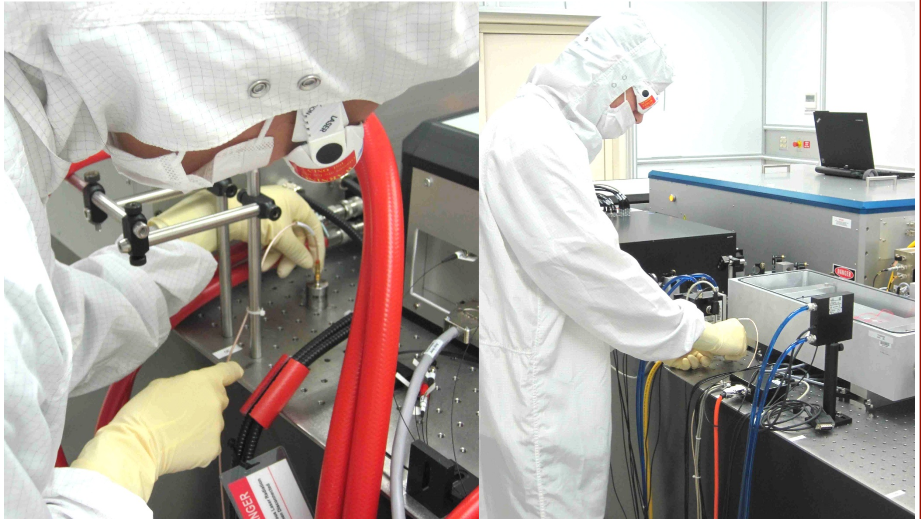
Terra and Vinny install accelerometers on PSL table
