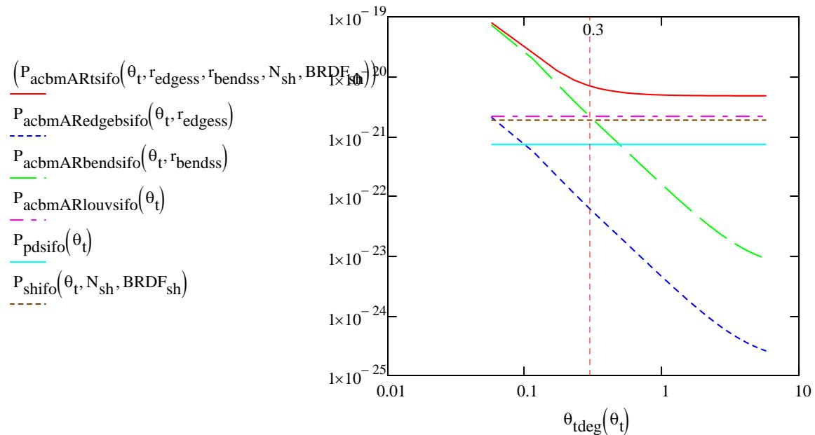
Note: the edge scatter does not dominate for tilt angles  $> 0.3$  deg
