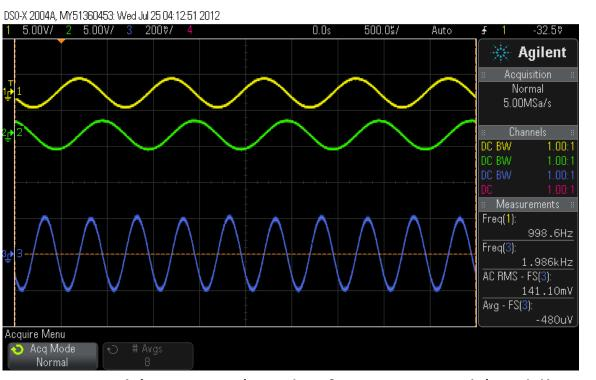
Input signal (top trace) and reference signal (middle trace ) of the same frequency and 90° out of phase. Output of hardware multiplier is the bottom trace. Note that the DC offset is zero and would result in an output that was nominally zero after passing through a low-pass filter.
