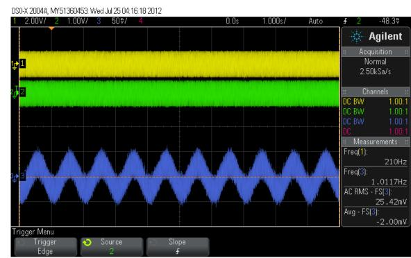
Input signal (top trace) and reference signal (middle trace ) of slightly different frquencies. (and on a Much expanded timebase). Students note that if this signal were low pass filtered, a beat frequency of 1Hz would result.
