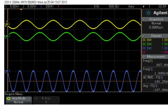
Input signal (top trace) and reference signal (middle trace) of the same frequency and 180° out of phase. Output of hardware multiplier is the bottom trace. Note that the DC offset is now negative.
