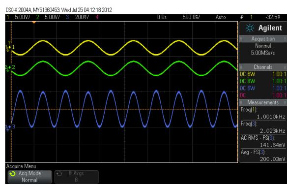
Input signal (top trace) and reference signal (middle trace ) of the same frequency and phase aligned. Output of hardware multiplier is the bottom trace. Note the DC offset - this is proportional to the input signal amplitude, the reference signal amplitude and the phase difference between them.
