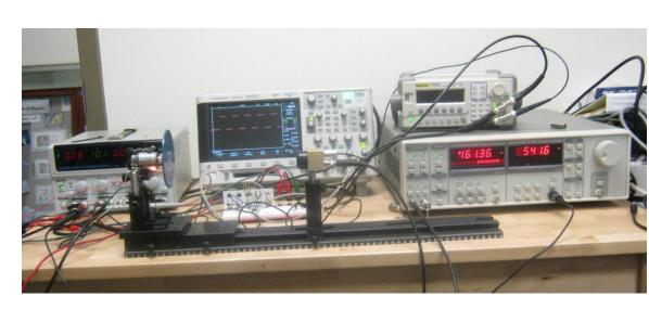
Lab station setup. Quad power supply is useful for supplying split power supply in addition to providing power for optical chopper and lamp. Breadboard with hardware multiplier can be seen behind optical rail.
