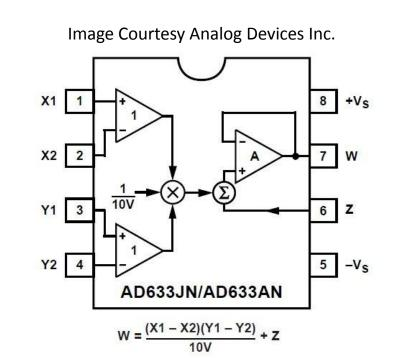
AD633 Four Quadrant Hardware multiplier. Useful for many of one's AC measurement needs!
