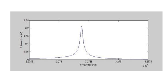
Crystal Q – the resonant peak of a tuning-fork watch crystal is gathered using a spectrum analysis LIGO Research – the normal modes of a suspended technique. Note the "parallel resonance" is not shown to avoid confusion.
