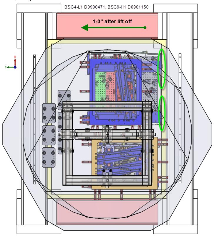
Circles in green indicate any protrusion into the keep out zone. Any global XY moves relative to the Test-Stand will depend on the orientation of the Test-Stand.
