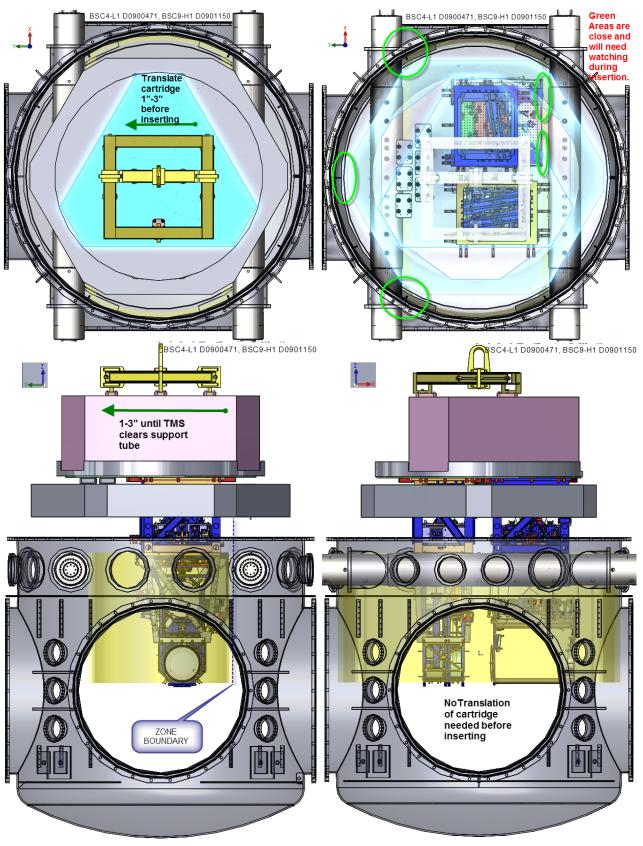
Locating the Bale pre-lift of the cartridge (Some adjustment will be needed)
