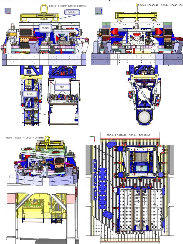
Cartridge installation of BSC. 3pt Lifting bar can cover the range of locations for the XY CG
