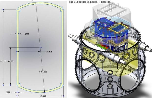
The Clearance Zone is a 2 inch wide area defined between the support tubes, and by the chamber shell. Any items on the cartridge that protrude partly into this zone should be considered for alteration or removal during install. ANY ITEMS THAT PROTRUDE ALL THE WAY INTO, OR THRU, THE ZONE, MUST EITHER BE REMOVED OR ALTERED SO AS TO STAY CLEAR OF THE ZONE FOR INSTALL.
