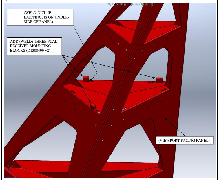
ABOVE: D1300499-v2 Pcal Receiver Mounting Blocks shown in place (to be welded) on an X-Arm pylon weldment D1001297. On Y-Arm pylon weldments D1001292, the arrangement is similar by symmetry.
