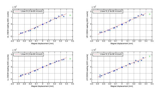
There are no requirements associated with this measurement. It is rather intended to be a sanity check looking for strange (e.g. non linear) behaviors and differences between OSEMs. **Passed**
