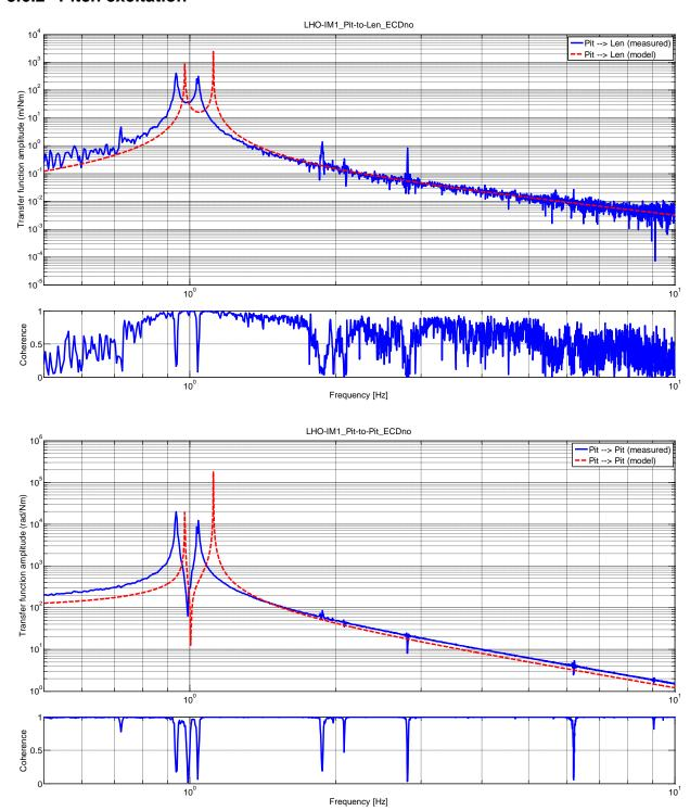
Possible double peak visible above 1Hz. However, the coherence in that region is low and there is no other indication of anomalies in the remaining TFs.
