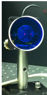
Figure 21: 2-inch CVI mirror with HR and AR coatings for 532 nm in a modified Newport U100-P mirror mount, on a 2.5-inch optical post.
