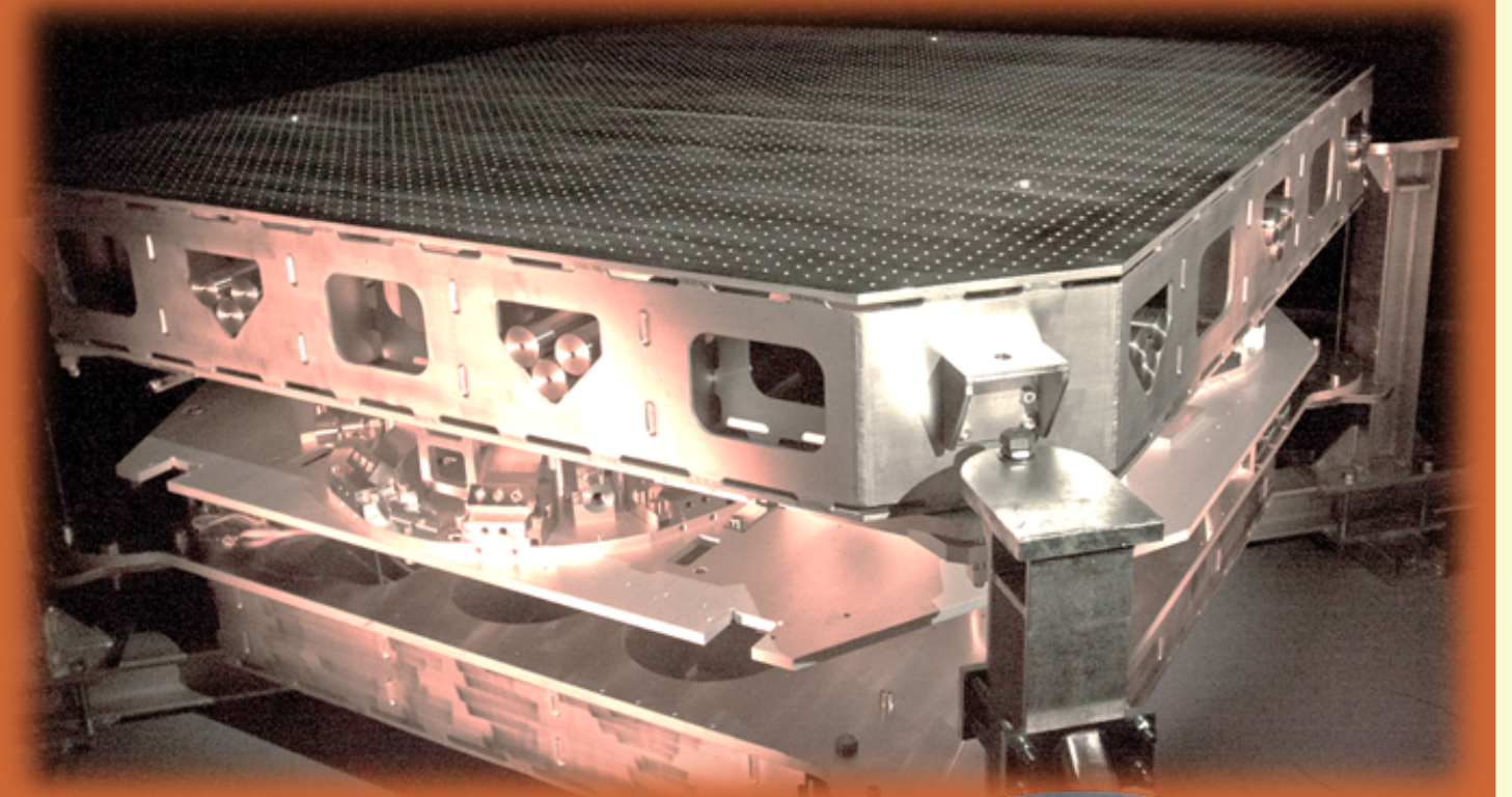
Two of three isolation tables are installed in the vacuum system
