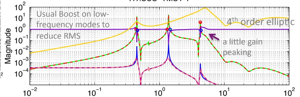
So, as with the vertical DOF in the Beam Splitter, I increased the order of the elliptic, and even added another (real) zero-pole pair at [0.6:25] to the roll-off to squeeze out as much phase as I could get...
