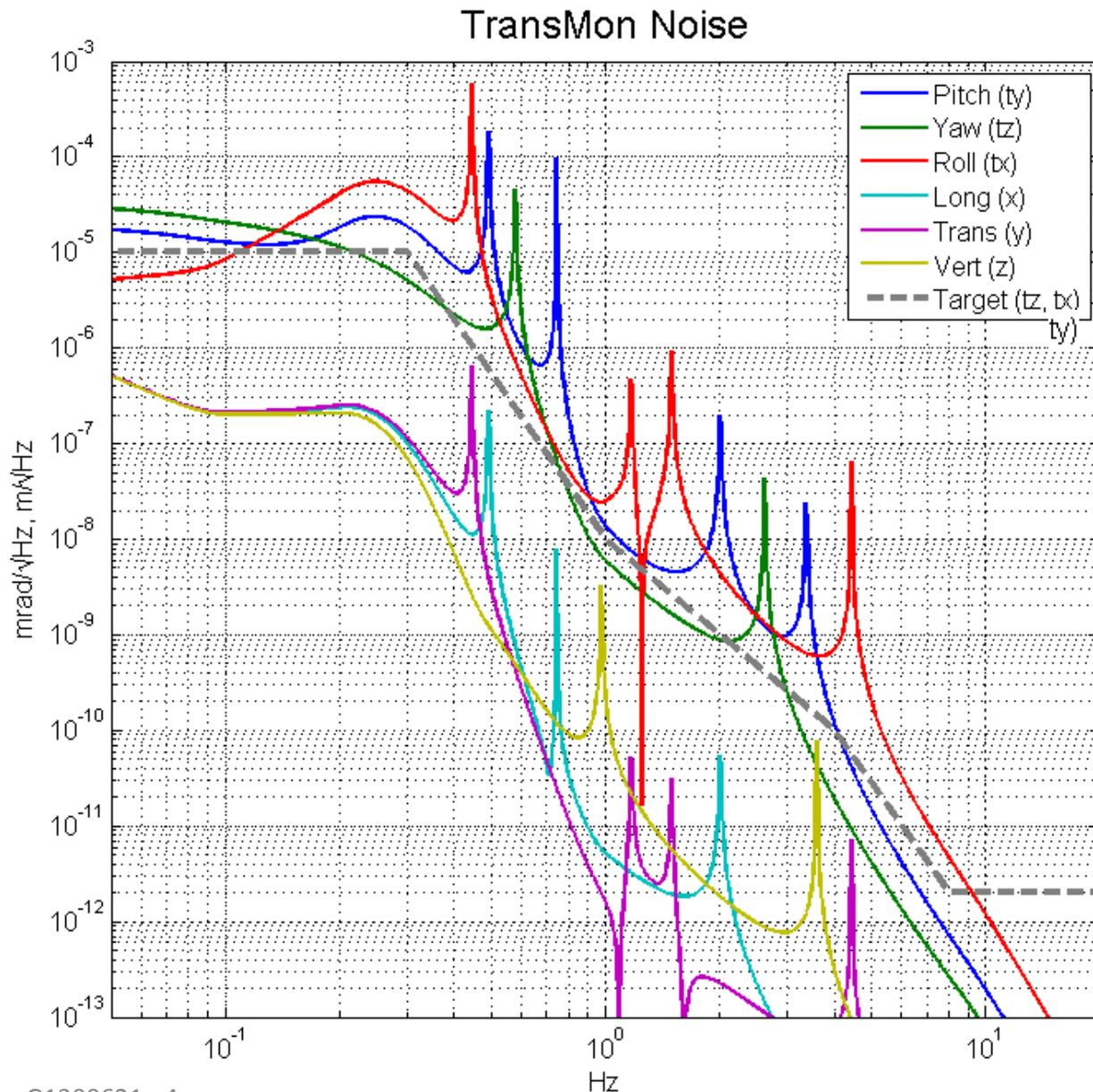
Original target for total displacement noise was based on **preliminary, SISO model of \*only\* residual seismic noise** (unclear why Roll was ignored)
