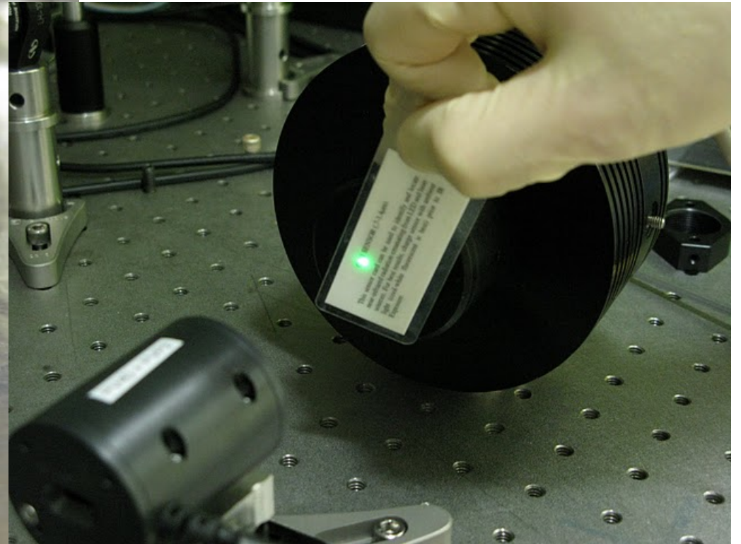
The green light generated from the crystal mounted in the oven
