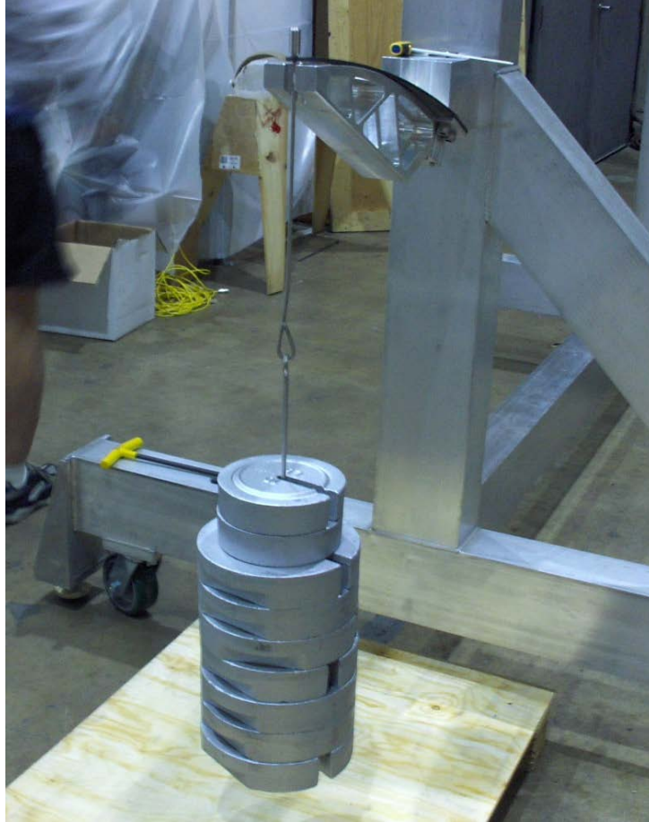
Figure 18: Pre Load Spring Blade by Hanging Weights
