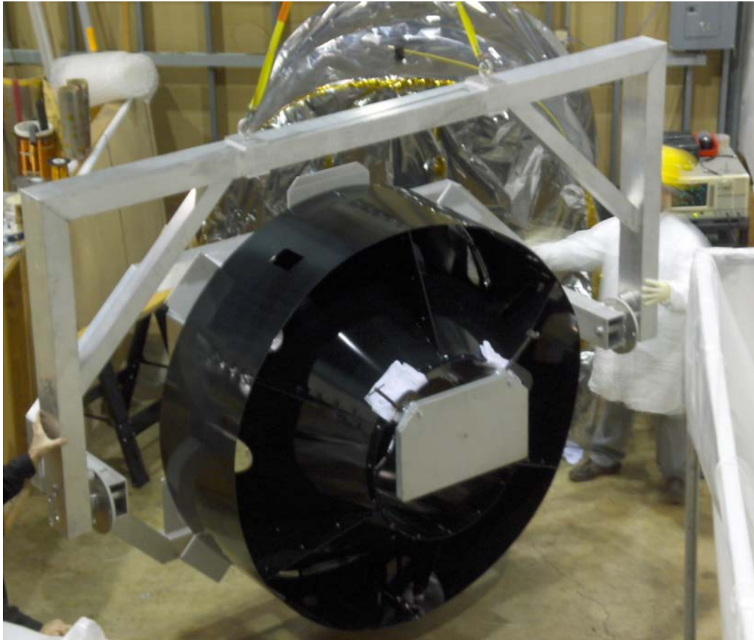
Figure 23: Lift/Assembly with Baffle Supported by Crane
