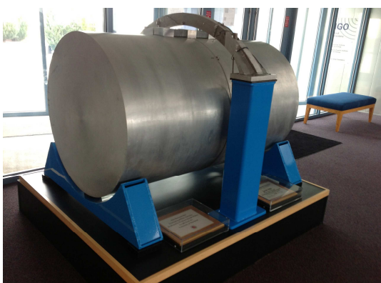
Figure 4: Weber bar at the entrance of the LIGO Hanford Observatory
