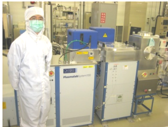
Plasmalab system100, Oxford Inst. Courtesy photo from National Nano-Device Lab (NDL) of Taiwan
