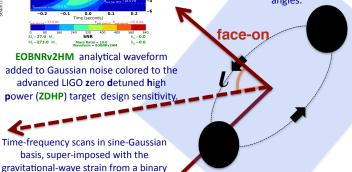
The amplitude of gravitational-wave strain is maximum when observed at the face-on direction. The strain amplitude decreases as the point of observation moves towards the edge-on direction.
