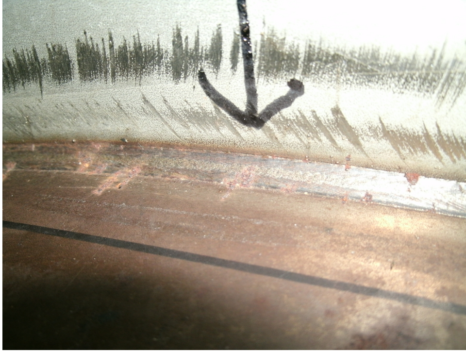
Figure 1: The location of the arrow is a likely place for the original leak on the continuous weld between the stiffening ring and the tube. The brown discolorations are assumed to be due to mouse urine.
