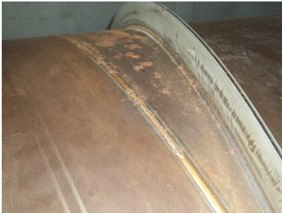
Figure 2: A larger view showing the stiffening ring and the spiral weld. The spiral weld is covered with mouse feces which comes off easily. The mouse urine has discolored the tube in patches between the spiral weld and the stiffening ring. The background brown color of the tube is due to the air heating of the tube material before fabrication to reduce the dissolved hydrogen in the steel.
