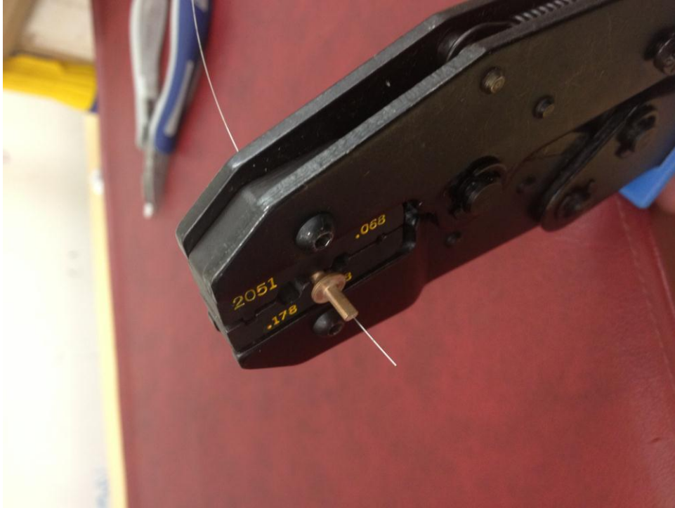
Figure 2. Crimping the clamp
