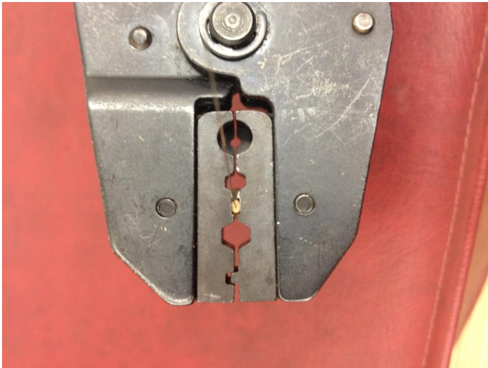
Figure 3. End view – not fully crimped yet
