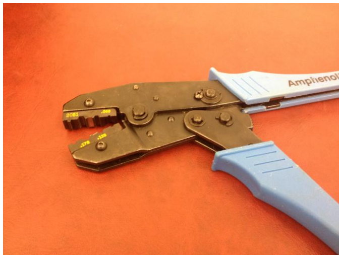
Figure 1. Modified Amphenol Crimpers → D1300083 (the blue handles were removed before C&B)
