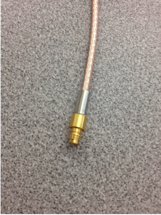
Figure (2) – (Above) Photo of proposed new cable connector (previously soldered joint)
