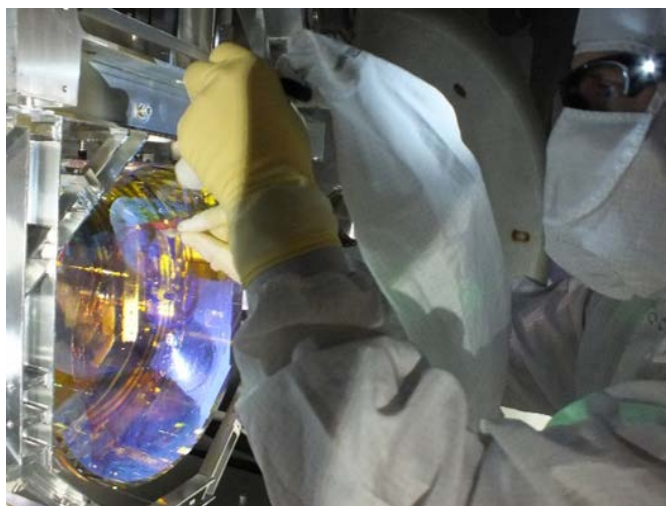
Figure 15. Pulling PEEK tab while using Top Gun
