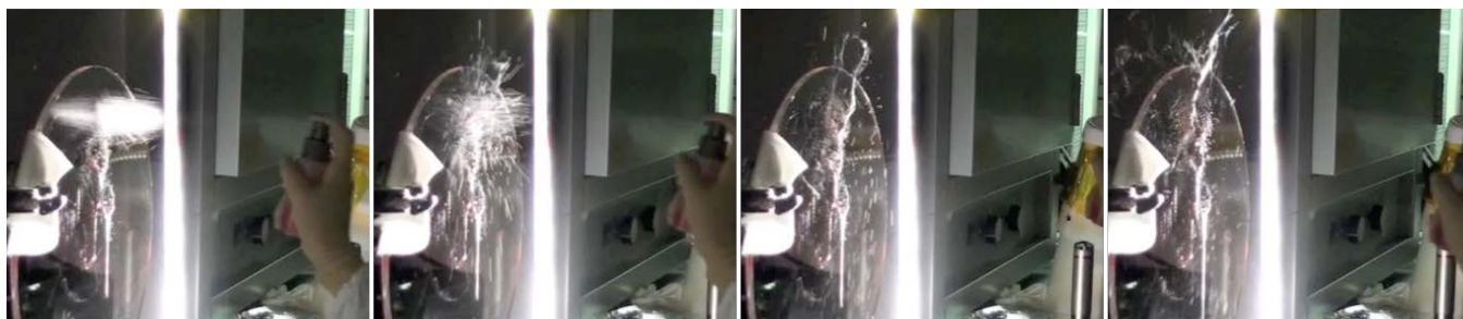
Figure 9. Creating of spider webs on glass plate
