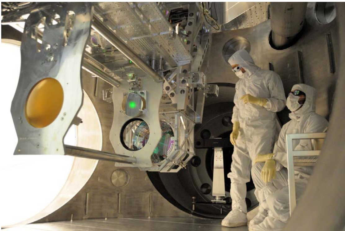
Figure 42: TMS Assembly being Installed in BSC
